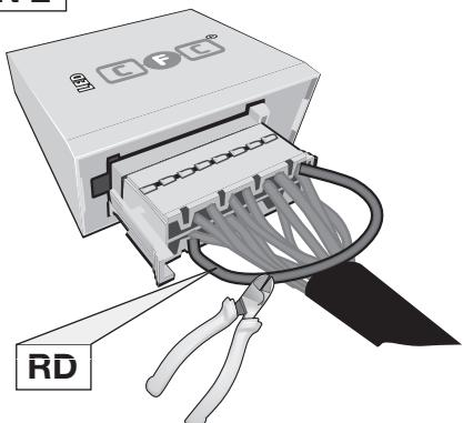
**Pin 11 and Pin 2 disconnected**
